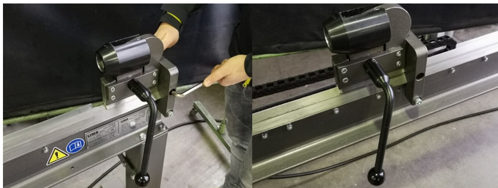
Fig. 18: Mounting the clamping head.
