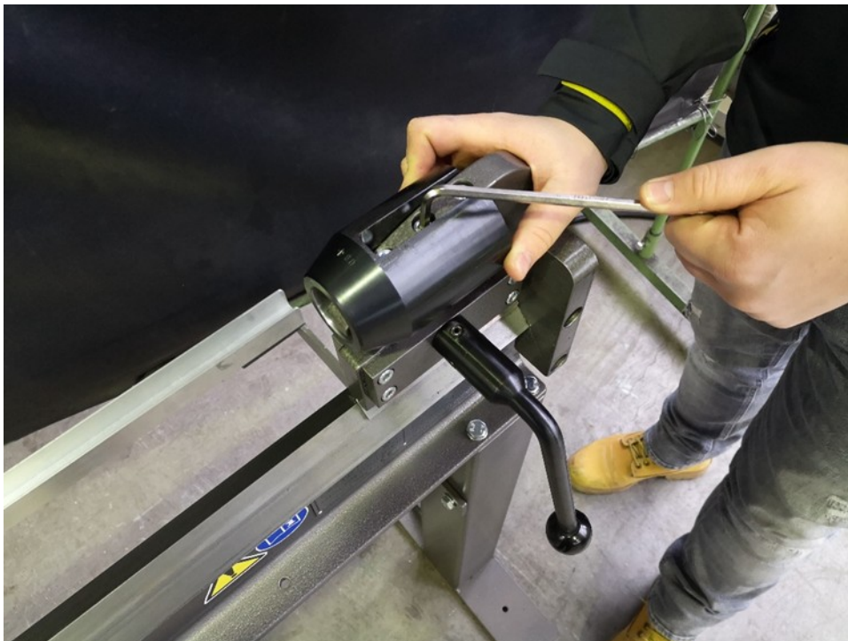
Fig. 16: Replacing the clamping head.
