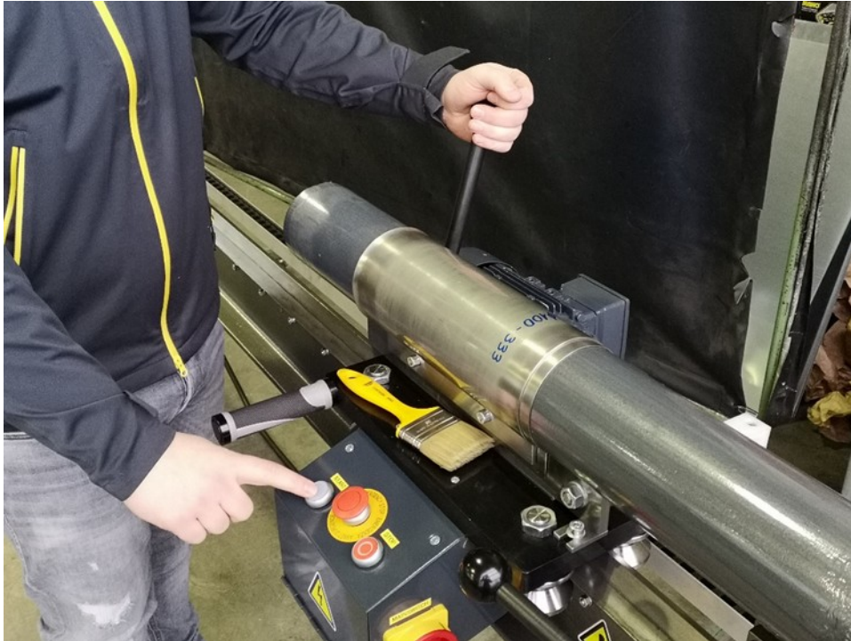
Fig. 12: Press the START button again after the pipe has been clamped to finish the pipe.
