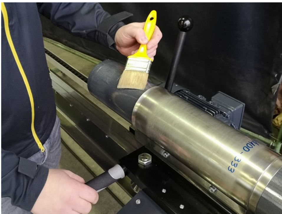
Fig. 13: Keep oiling the pipe for smoother seaming.
