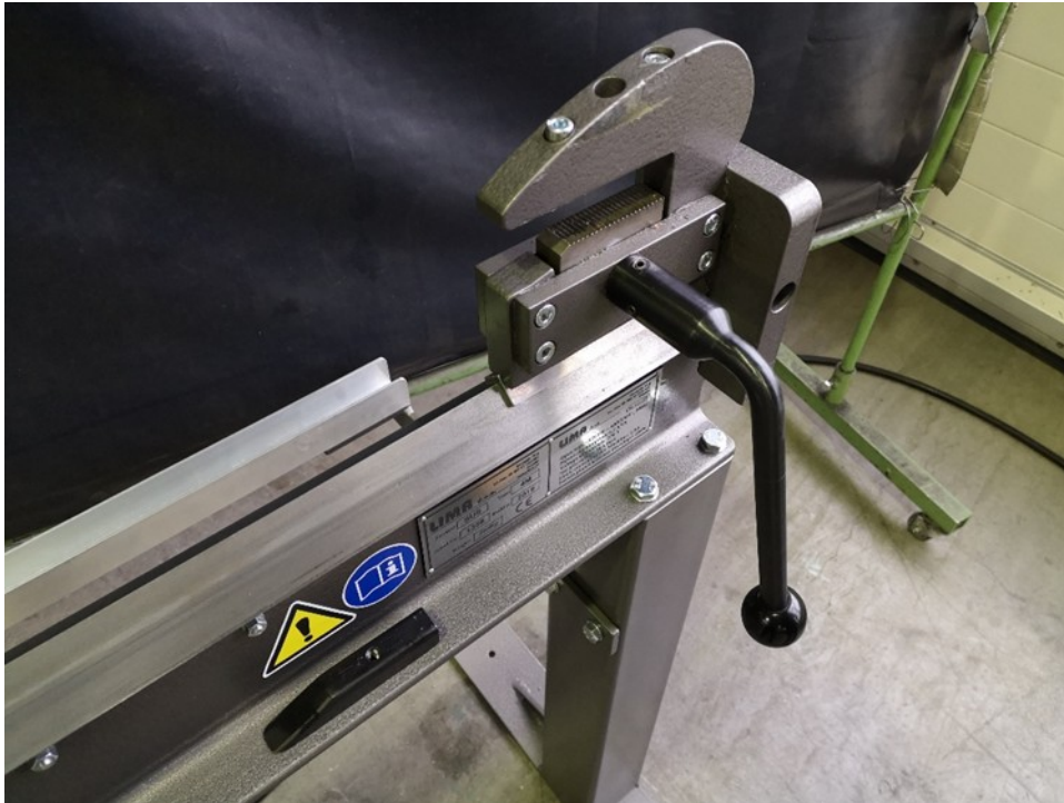
Fig. 17: The clamping head holder without the clamping head attached. Visible in the lower left is the clamping attachment for non-round pipes.
