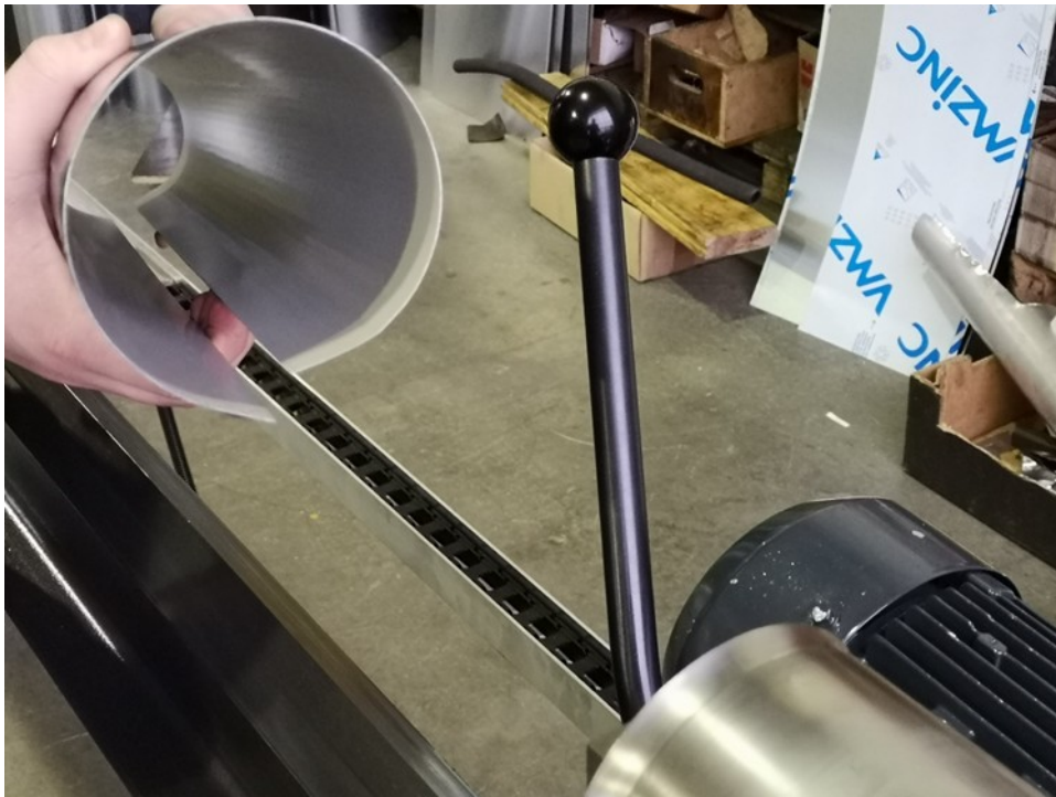
Fig. 3: The correct position of pre-shaped pipe ends, with the end on the side of the engine being higher. This way the pipe will be seamed correctly.
