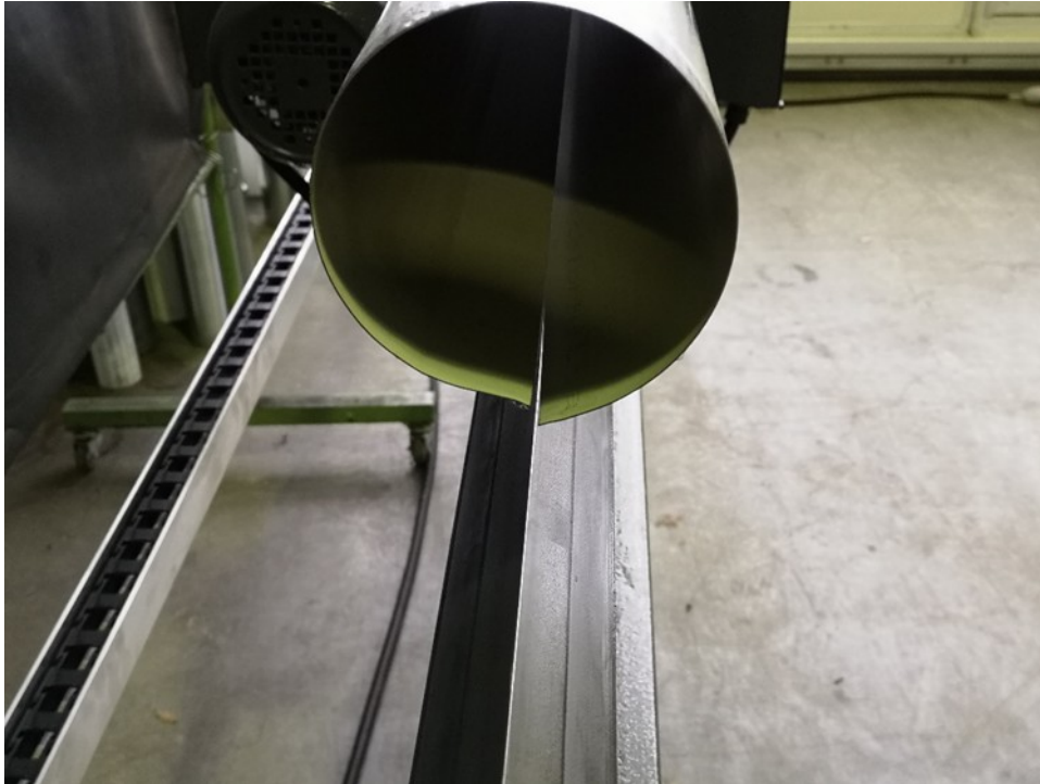
Fig. 6: The correct pipe placement over the guide rail, with the overlapping pre-shaped pipe edges being directly above the guide rail top edge.
