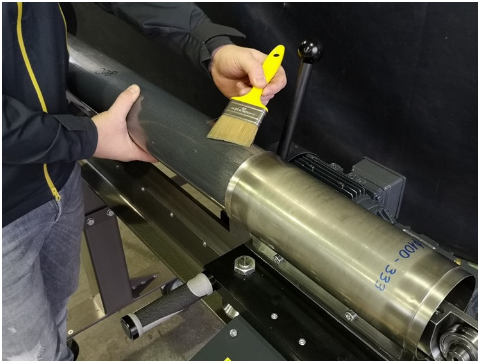
Fig. 9: Apply oil as the pipe enters the seaming head.
