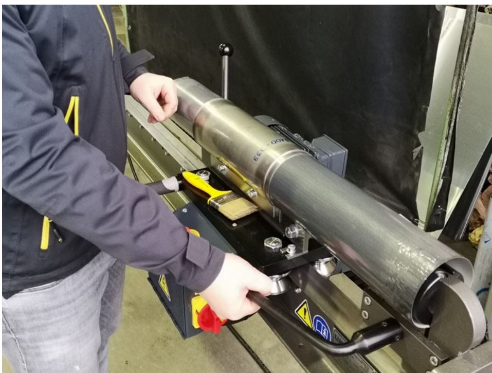
Fig. 11: Pipe clamped in the clamping device.
