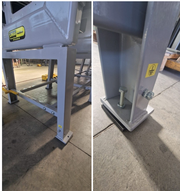
Fig.2 Grounding clamp, on the right most leg of the machine.
