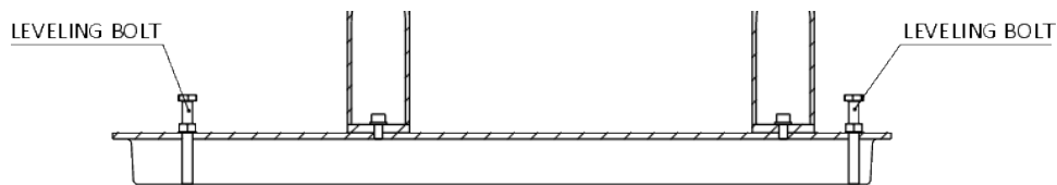
UNP profile with leveling bolts shown.
